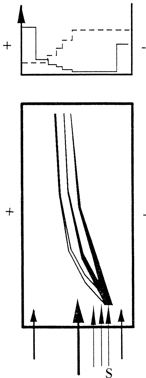
Fig. 4. Scheme of ITP. Anodal margin buffer, leader medium (bold arrow) spacer fluids and terminator medium (=cathodal margin buffer) are introduced into the chamber as indicated. S indicates the sample dissolved in the most cathodal spacer medium. The small upper scheme shows the pH (dashed line) and conductivity (solid line) profile obtained by analysing the buffer leaving the chamber.
